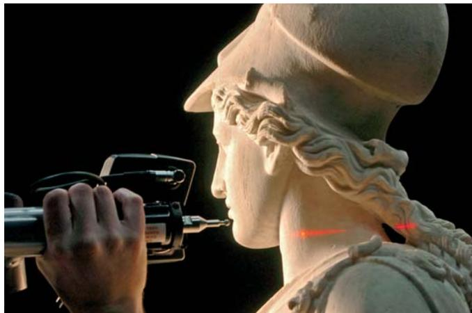
3D recording using non-contact laser scanning.
